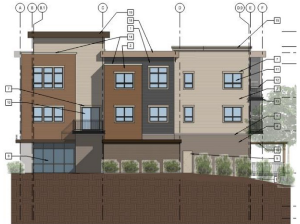
Roof parapet used to screen rooftop mechanicals
