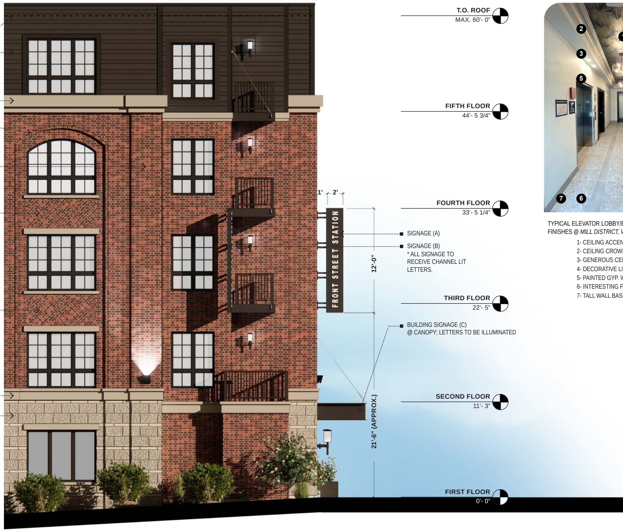
1 ENLARGED BUILDING ELEVATION | TYPICAL EXTERIOR BUILDING MATERIALS & SIGNAGE DESIGN SCALE: N.T.S.
