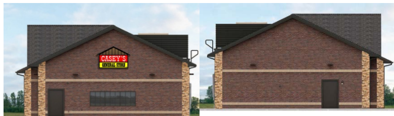
Metal screening of rooftop mechanicals
