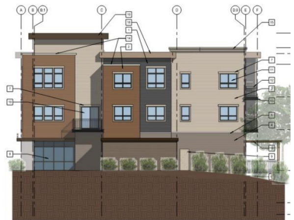
Roof parapet used to screen rooftop mechanicals
