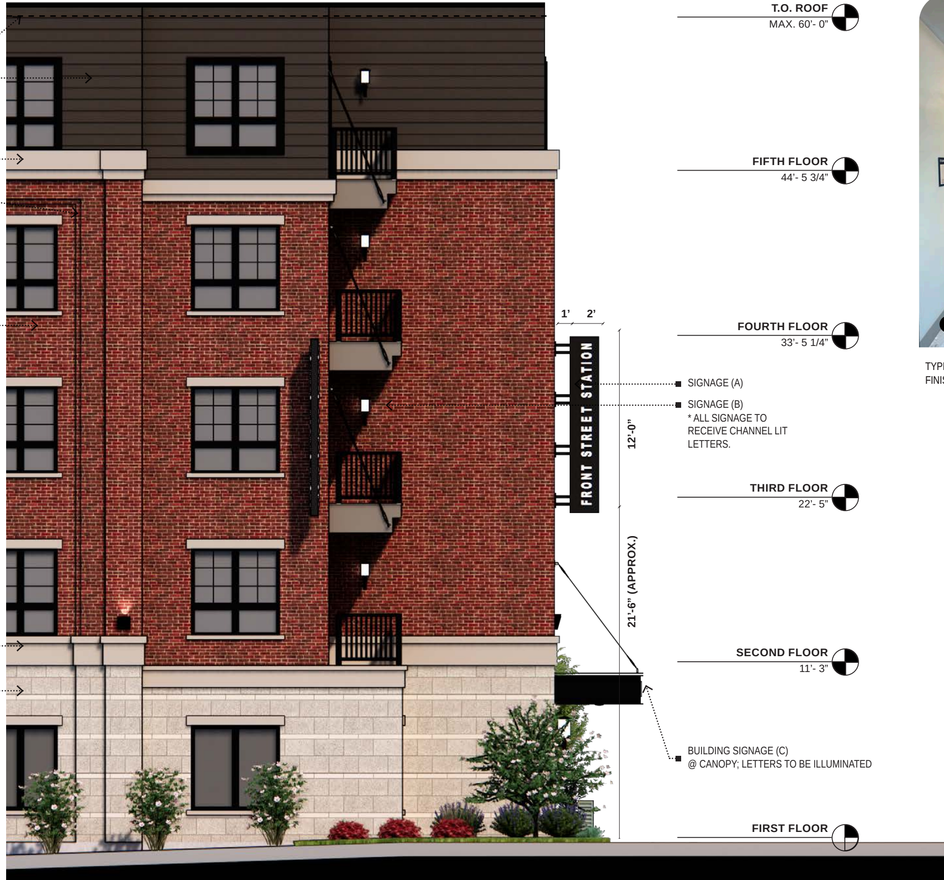
1 ENLARGED BUILDING ELEVATION | TYPICAL EXTERIOR BUILDING MATERIALS & SIGNAGE DESIGN SCALE: N.T.S.
