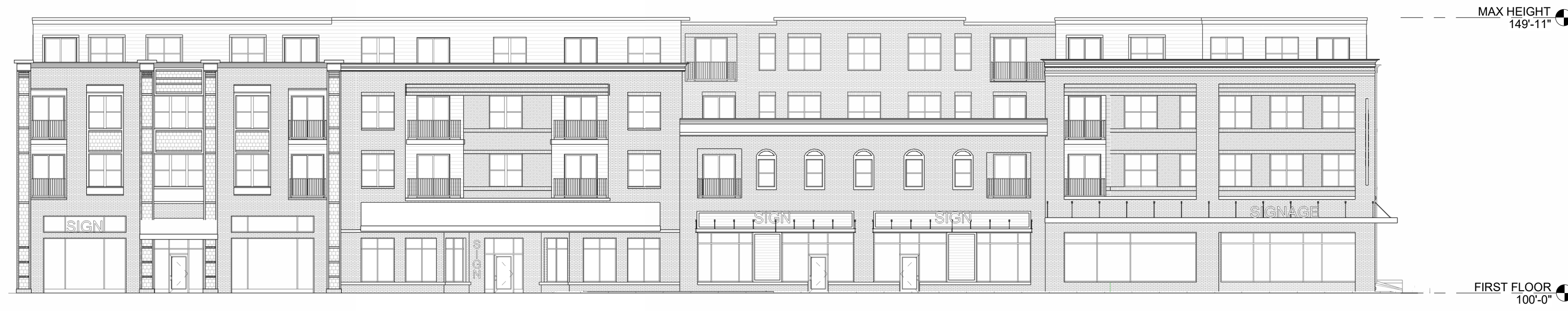
3 SOUTH ELEVATION - B&W 1/16" = 1'-0"
