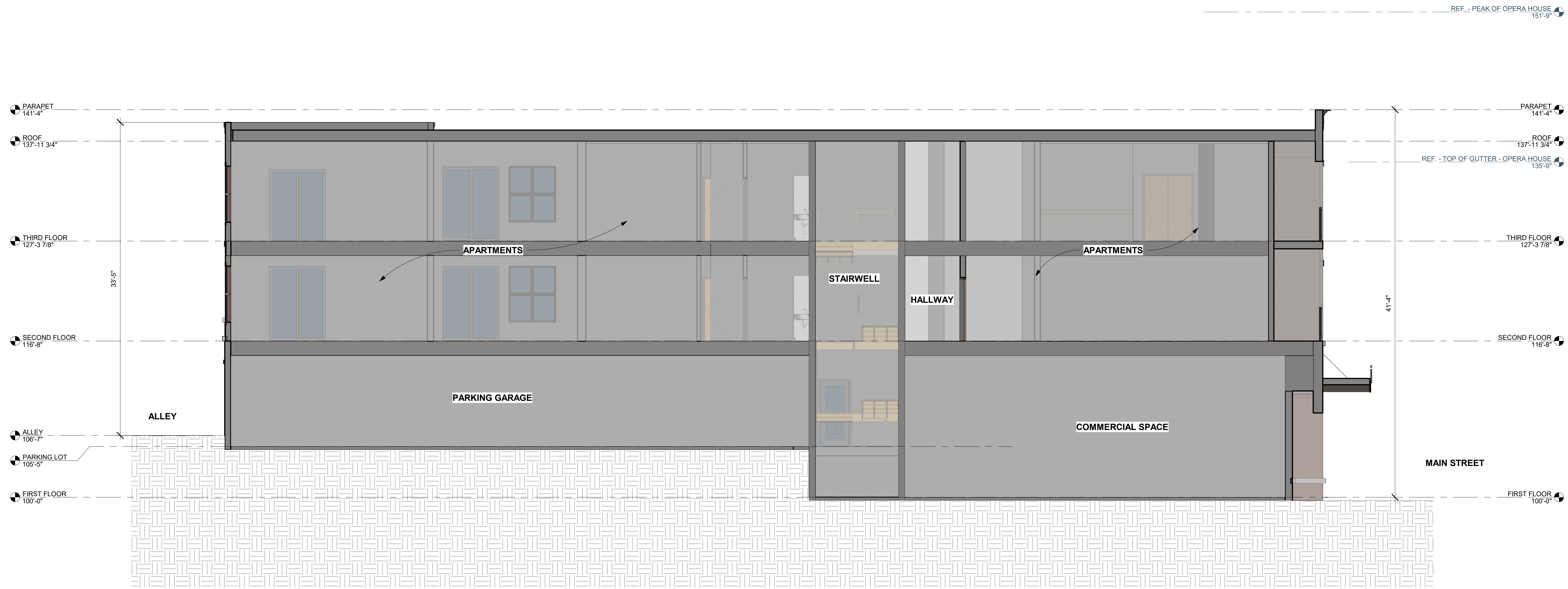
BUILDING SECTION - GRADE CHANGES
