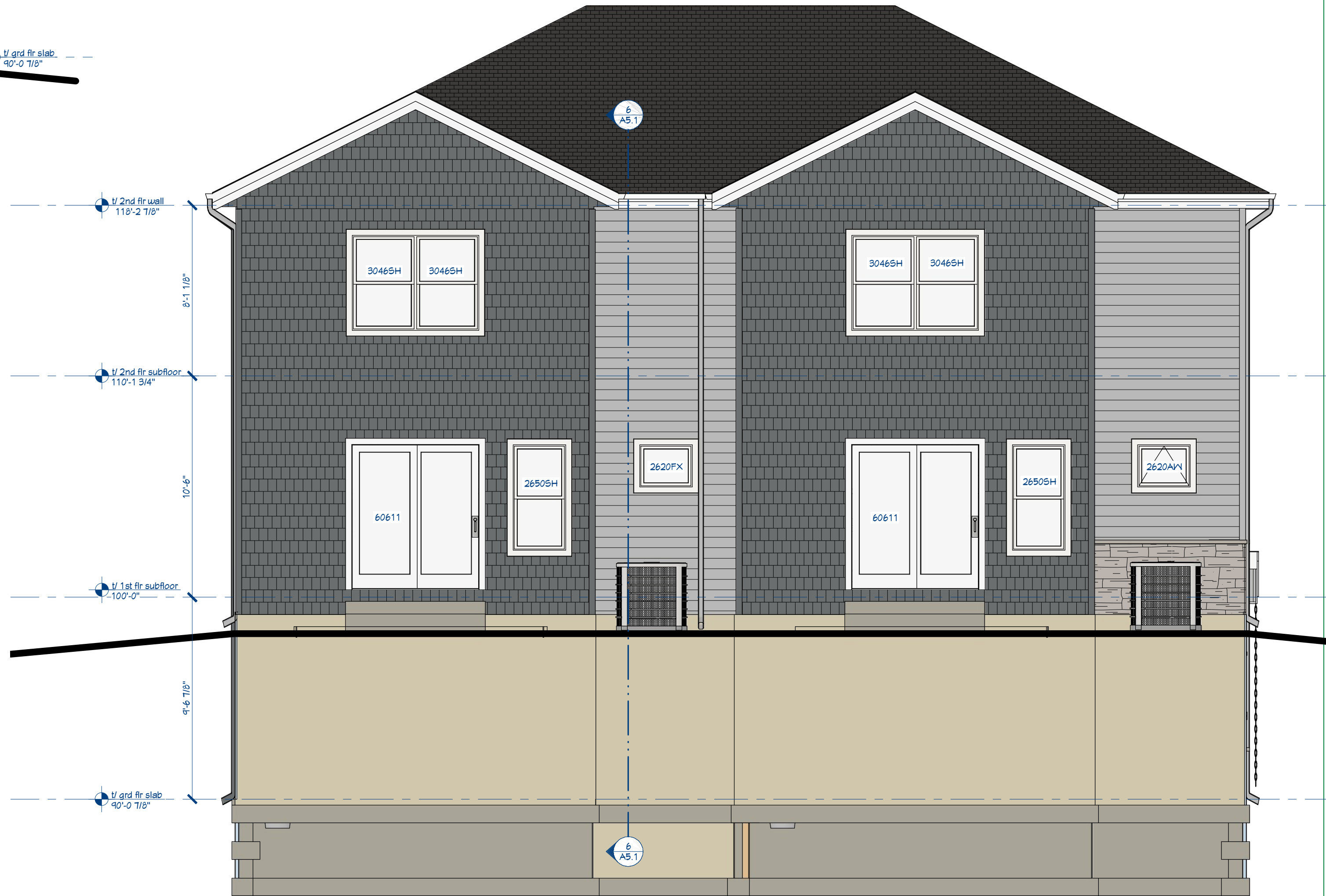
2 Exterior West Elevation SCALE: 1/4" = 1'-0" (22"x34" - Full size) 1/8" = 1'-0" (11"x17" - Half size)
