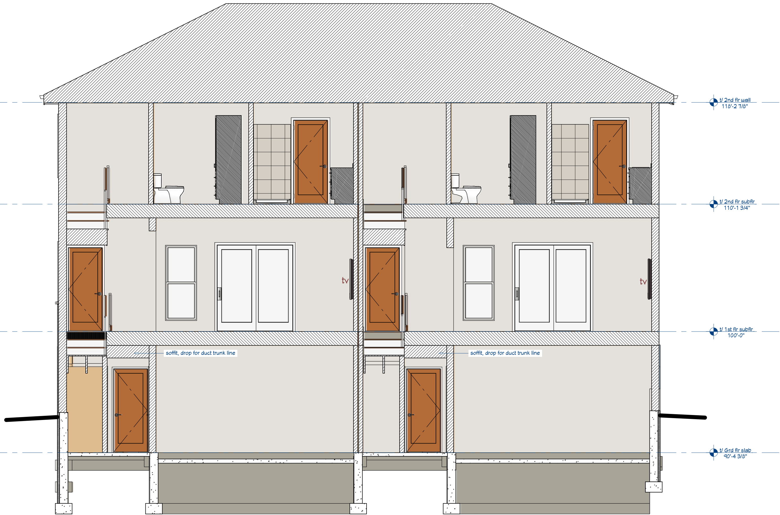
1 Building Section SCALE: 1/4" = 1'-0" (22"x34" - Full size) 1/8" = 1'-0" (11"x17" - Half size)
