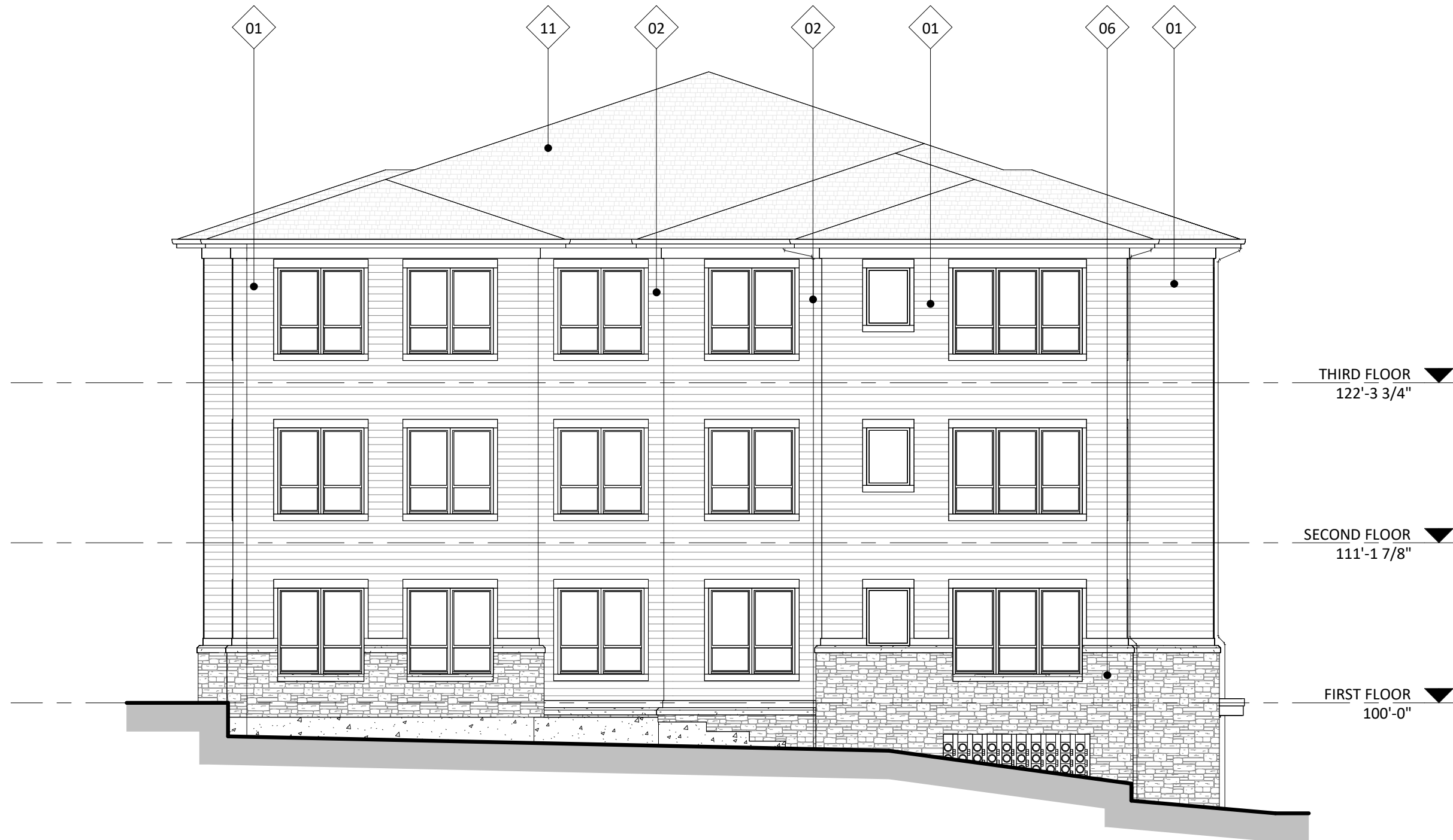
2 NORTH ELEVATION AC201.2 1/8" = 1'-0"
